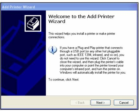
c. For Local or Network Printer, click the Local printer attached to this computer radio button, and uncheck Automatically detect and install my Plug and Play printer. Click Next.
