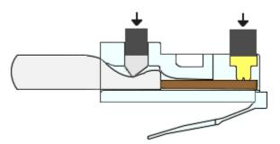
d. Visually re-inspect the connector. If improperly installed, cut the end off and repeat the process.
