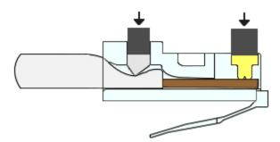
d. Visually re-inspect the connector. If improperly installed, cut the end off and repeat the process.
